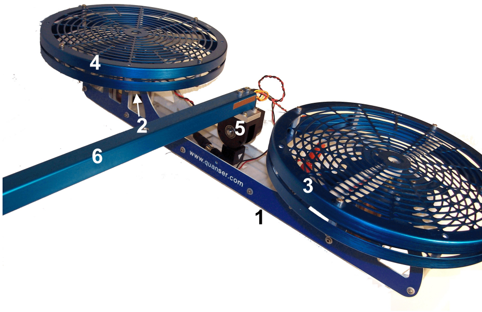
Figure 5: Components on the helicopter body of the 3-DOF Helicopter system.
