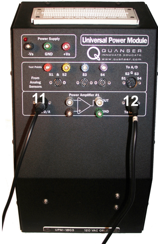
Figure 20: Connections on UPM-1503 used for ADS motor.
